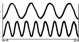
distance between points A and B represents one second, the upper wave goes through four cycles a second, while the lower goes through eight cycles per second. The upper has a frequency of 4 hertz (Hz), while the lower has a frequency of 8 Hz.
